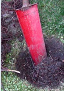
A soil sampling probe, auger or shovel can be used to collect soil samples. Remove surface vegetation before collecting the sample.
